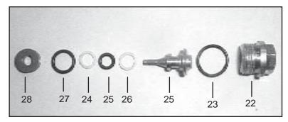
7. Remove the piston (24), o-ring (26), and backup rings (25). Remove the bypass valve seat (28). Inspect the parts for wear and replace as necessary. IMPORTANT! Make sure that the shoulder on bypass valve seat (28) is facing the discharge plug (22).
