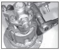
6. With a 14mm socket wrench, remove the guide plug (22) and o-ring (23).
