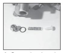
Remove the valve spring (18) and valve cone (36) from the manifold (35). Inspect the parts for wear and replace as necessary.
